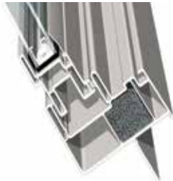
BarrierXP iE features carbonized foam liners in select masterframe channels for increased energy efficiency.
